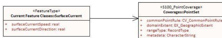
Figure B-7-3 – Example of coverage feature and type elements conforming to S-100 (from S-111)
