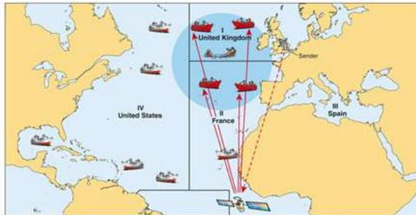
Figure 5 – SafetyNET message addressing to a circular area
