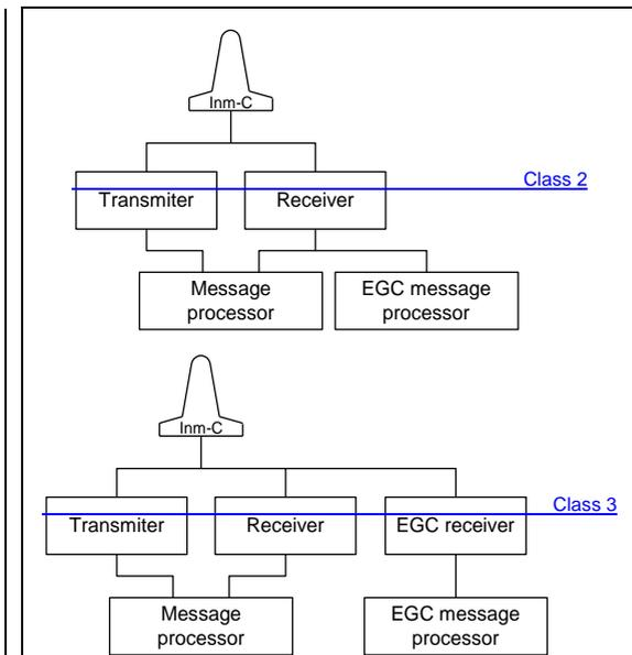
Figure 910 – Classes of [Inmarsat-C](#)/[Inmarsat C](#) Mobile Earth Stations
