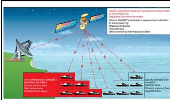
Figure 2 – Basic concept of the Inmarsat Enhanced Group Call system
