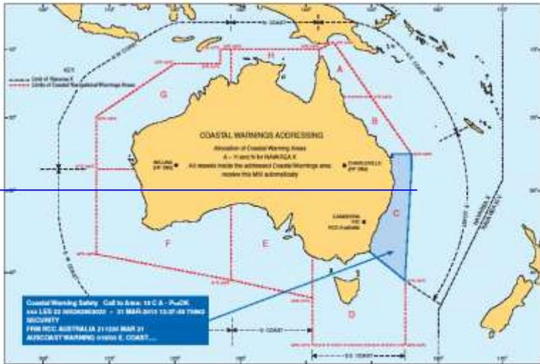
Figure 7 – SafetyNET message addressing to a coastal warning area
