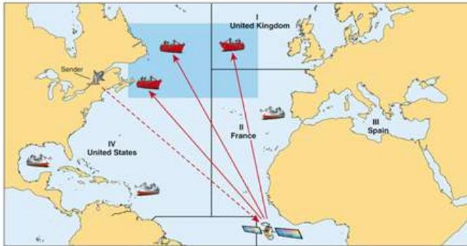
*Figure 6 – SafetyNET message addressing to a rectangular area*
