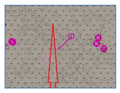
$\underline{Possible\ solution} \hbox{: As\ suggested\ in\ UOC\ (\S 5.8.2)\ DEPARE\ objects\ can\ be\ encoded\ with\ a\ CTNARE\ and\ appropriate\ value\ of\ QUAPOS\ on\ bathymetric\ objects.}$
