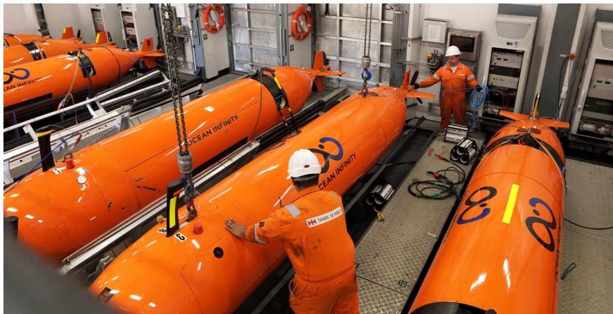
Figure 8: Ocean Infinity's AUV's being prepared to autonomously map the ocean floor, aboard Seabed Constructor
