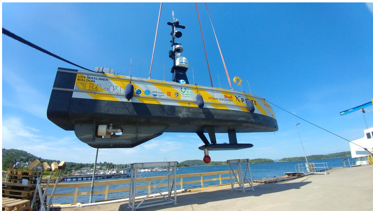
Figure 4: The USV Maxlimer is a remotely controlled surface vessel built by Hushcraft in the UK and is part of the GEBCO-Nippon Foundation Alumni Team's entry for the Shell Ocean Discovery XPRIZE. It has the ability to remotely launch and recover an Autonomous Underwater Vehicle (AUV) thereby reducing costs for obtaining high quality bathymetric data.
