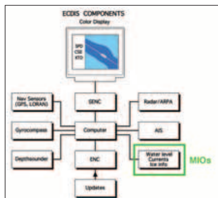
▲ Figure 1: ECDIS components
