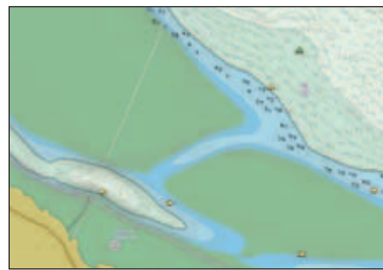
▲ Figure 3: SevenCs example of a time sequence of 'tide-adjusted ENC' showing changes that occur for depth areas
