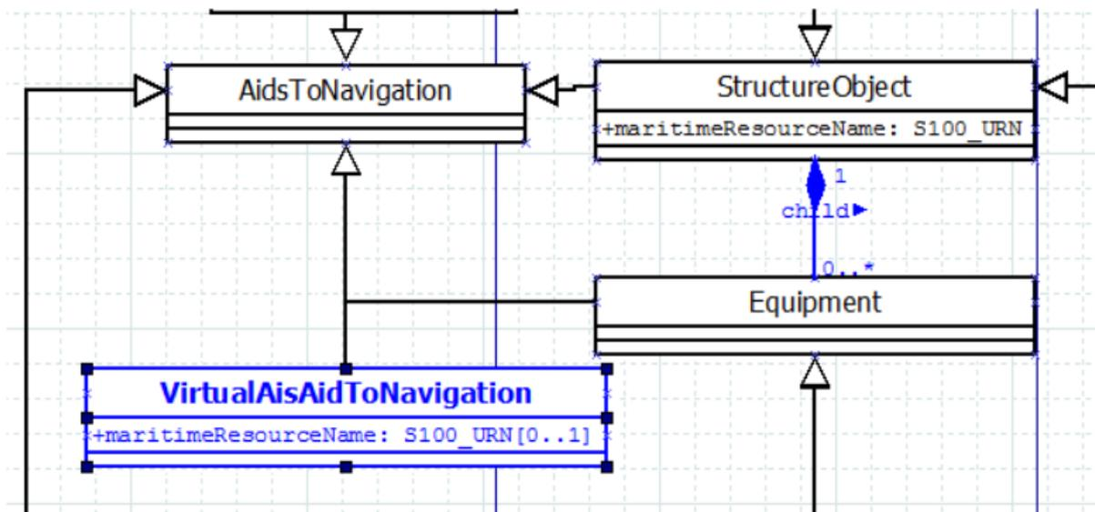
Figure 1 Addition of MRN to the structure- and VirtualAisAidToNavigation features.
