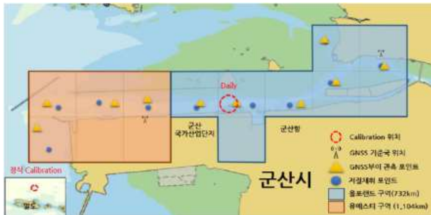
Fig. 2 S-102 Coverage of creating test datasets of S-102 Bathymetric surface grid
