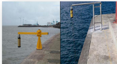
Figure 12, Microwave tide gauge recently installed along Egyptian coast
