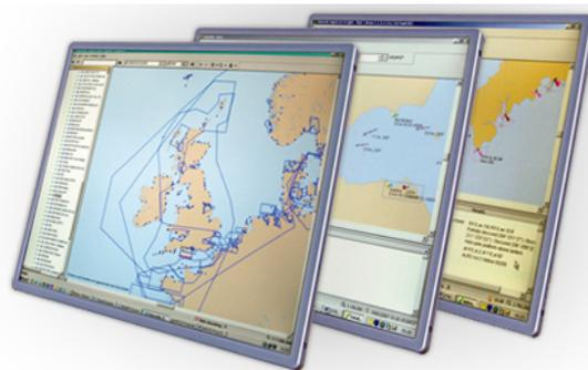
**4.2** The UKHO continues to develop digital equivalents to its existing paper publications, to support the IMO mandation of ECDIS; these publications have advantages to the mariner of providing additional functionality and minimising the task of updating.
