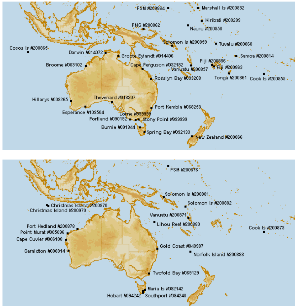
Fig. 3: Australian Baseline and South Pacific SEAFRAME stations (top) and additional ATWS radar gauges (bottom) used for monitoring of tsunamis in the Australian region.
