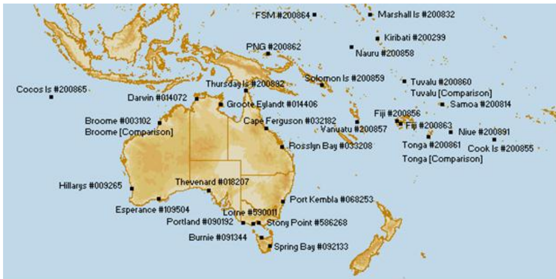
Figure 1 Permanent tide gauge network operated by the Bureau of Meteorology, including the Australian Baseline Sea Level Monitoring Array (16 sites) and Pacific Sea Level Monitoring Project (14 sites).
