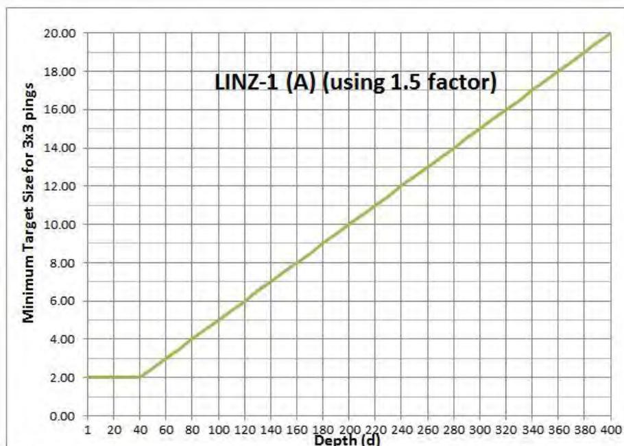
**Figure 17.** Target Detection Criteria for LINZ-1
