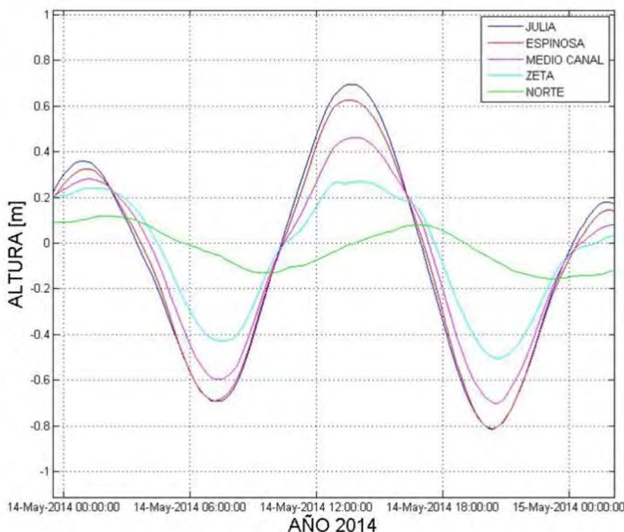
**Figure 4.** Tidal wave observed between 14<sup>th</sup> and 15<sup>th</sup> May. An asymmetric distortion can be seen in the tidal waves in Isla Zeta and Isla Norte sensors.
