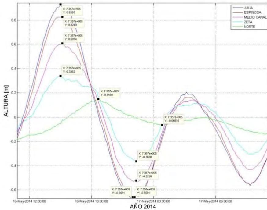
**Figure 6.** Tidal wave registered with maximum and minimum height values for each sensor defined as variable "y" (16<sup>th</sup> and 17<sup>th</sup> May)
