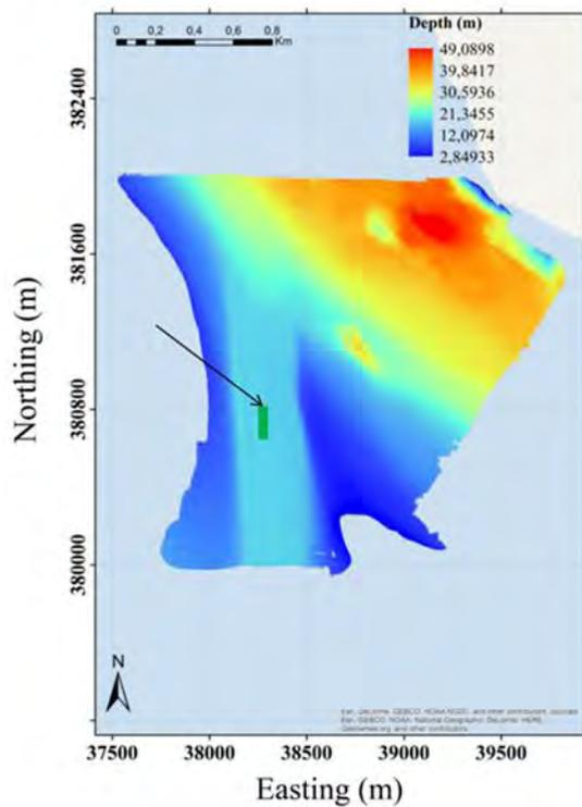
**Figure 2.** Bathymetry map of the area B in the Westerschelde estuary. The green thick line indicates the location where the seafloor profile is obtained (see Figure 9).
