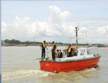
Side Scan Sonar Operation using NIMROD Motor Boat
