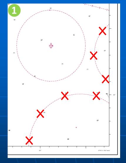
**1** Avoid representing swinging circles that partially fall into the chart, unless the point of the anchor berth falls within the chart borders.
