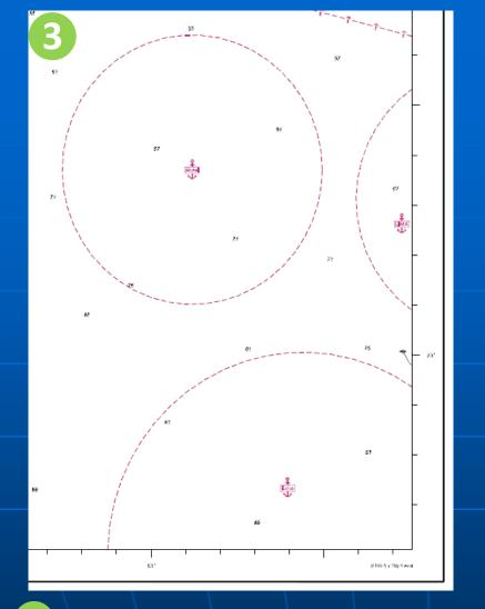
**3** Force the anchor berth symbol N 11.1 into the sector of swinging circle partially shown into the chart.
