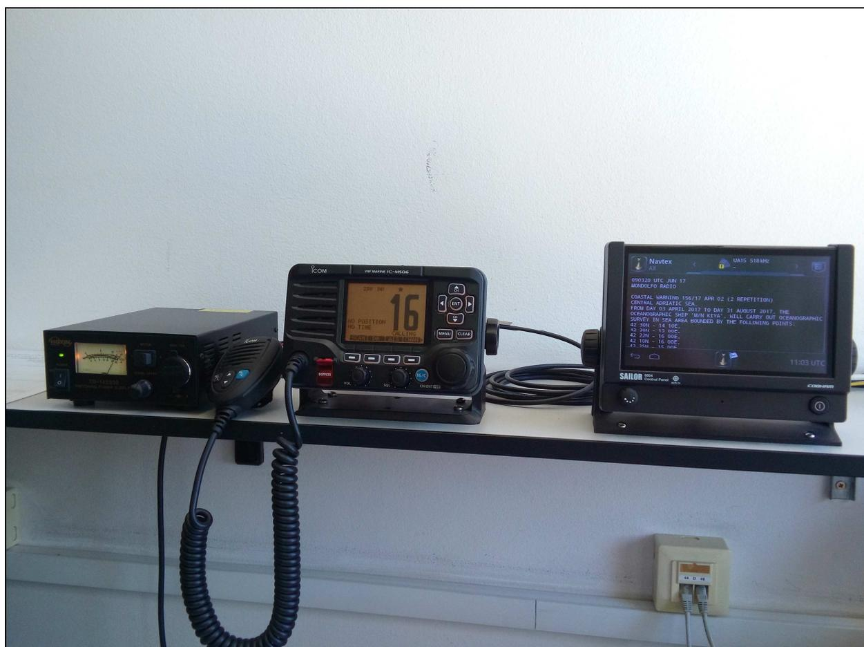
Figure 4. Equipment for monitoring the correctness of the promulgation of navigation warnings
