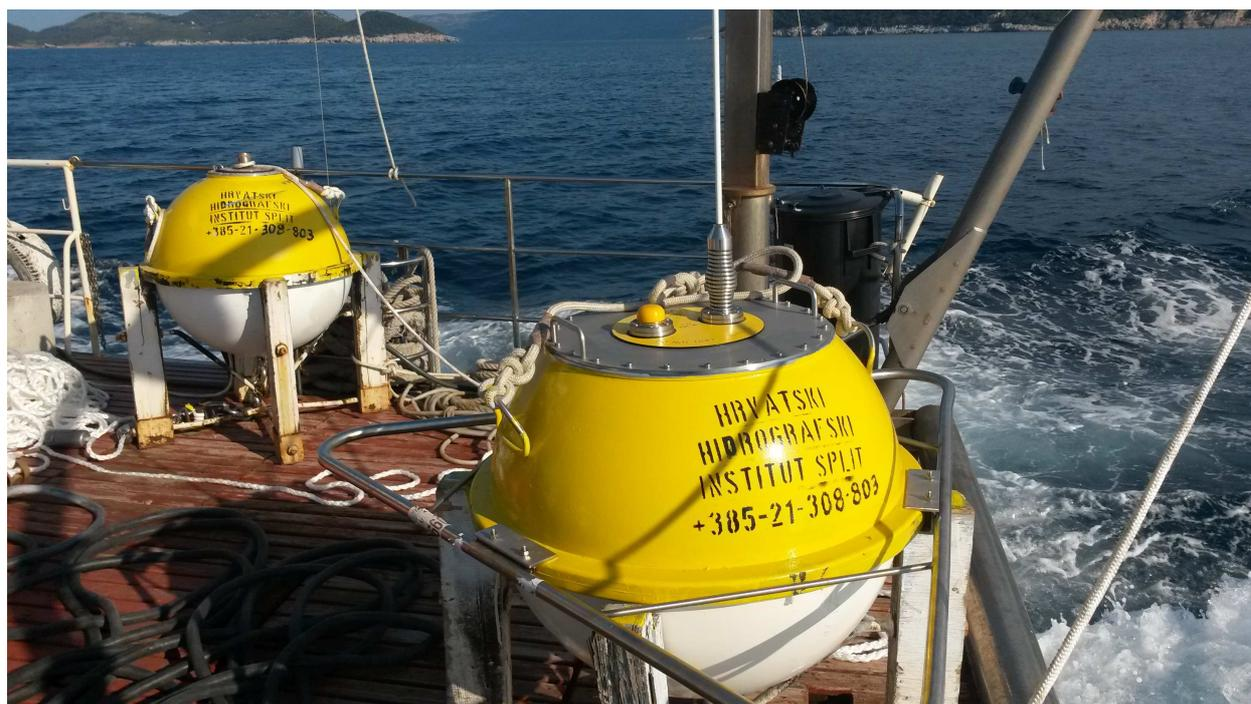
Figure 17. Directional wave rider buoy
