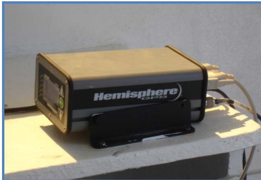
GPS Receiver Unit: The Crescent VS-100 GPS receiver is currently held in place in its mounting brackets with only two (2) screws rather than four (4) screws as stated in the operating manual.
