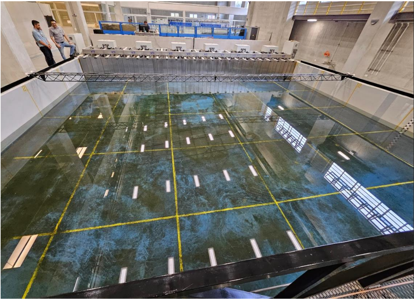
Image 5 Model at UCR which iMARES uses to conduct study of waves on breakwaters
