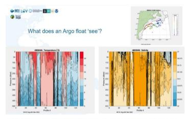
In Argo float can "see" temperature and salinity at different depths @ Argo
