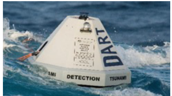
DART® - ETD (Easy to Deploy) buoy system Deep Ocean Assessment of Tsunami (DART), Source: NOAA, https://nctr.pmel.noaa.gov/Dart/
