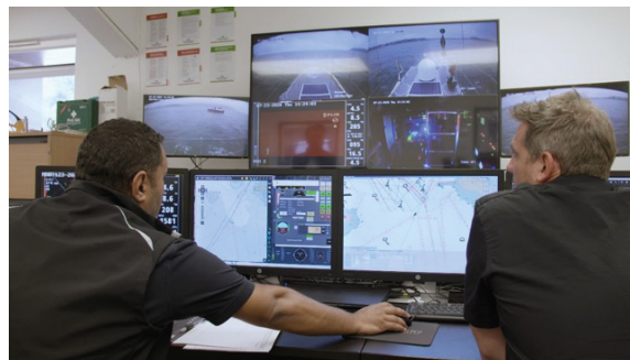
Source: SEA-KIT International and SEABED 2030, Seakit remote control of survey operations.
