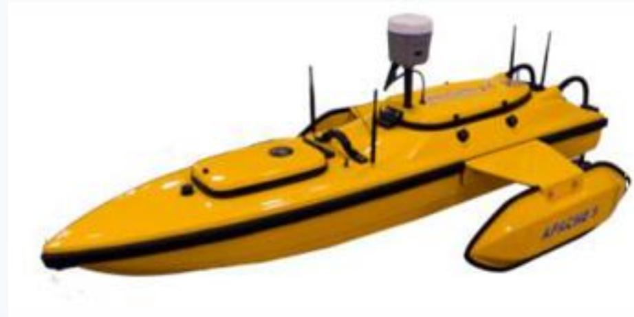
Unmanned surface vehicle – Multibeam survey
