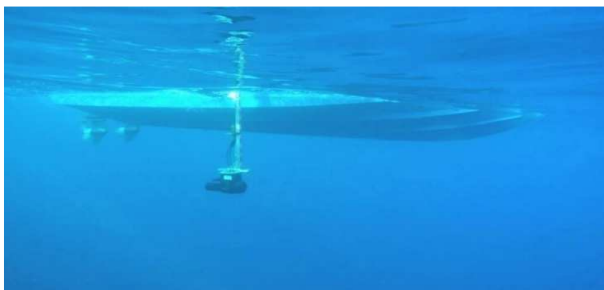
MBES Norbit iWBMSH integrated to Shom's deployable hydrographic system
