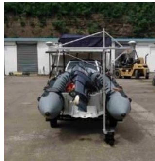
MBES Norbit iWBMSH integrated to Shom's deployable hydrographic system
