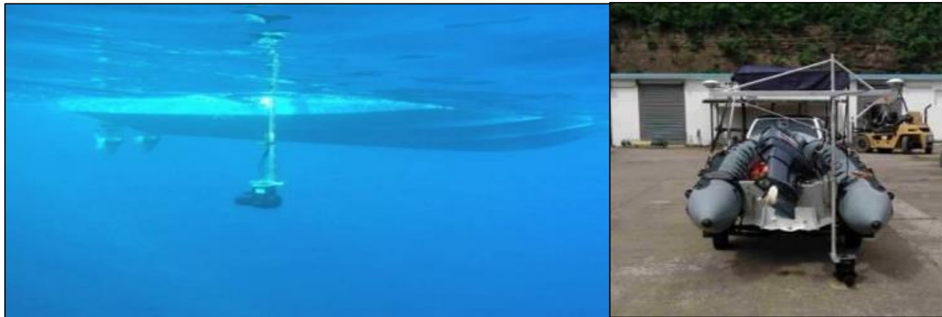
MBES Norbit iWBMSH integrated to Shom's deployable hydrographic system
