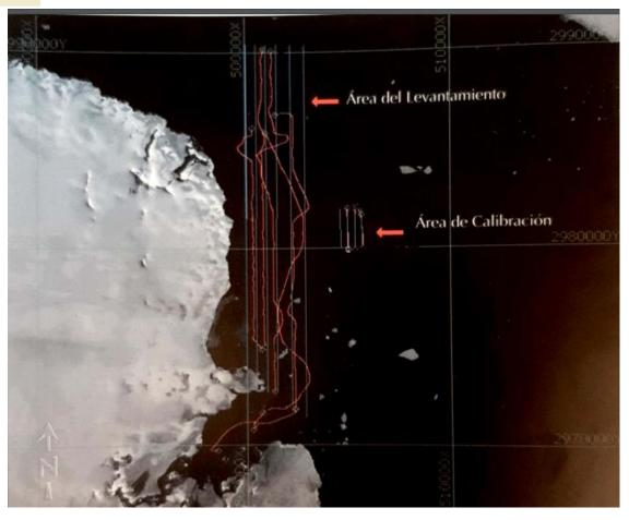
Esperanza Bay-Antarctic Strait Single beam bathymetry surveyed the february 2008.
