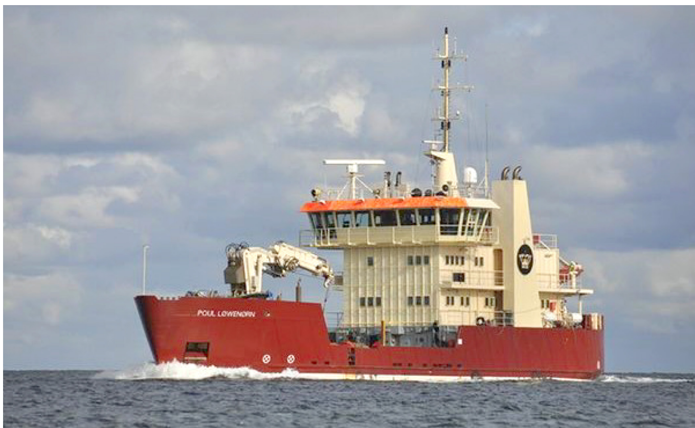
Figure 4: POUL LØWENØRN was fitted with two new cabins, a larger mess and was built 5 meters longer.
