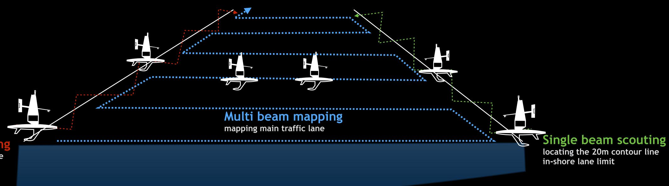
Single beam scouting locating the 50m contour line in-shore lane limit
