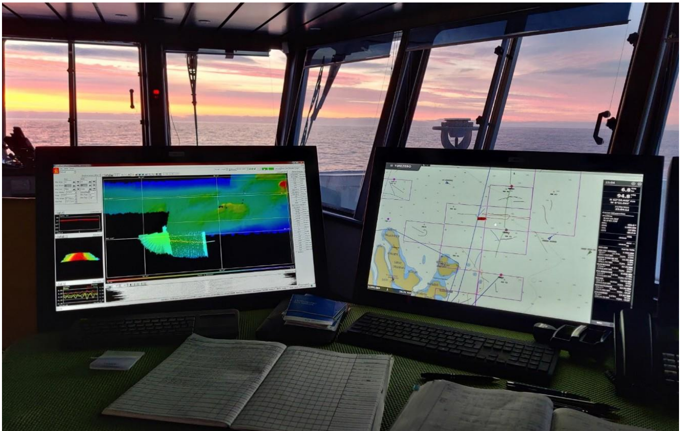
Figure 9: Image of the EM712 in action using Kongsberg SIS software.
