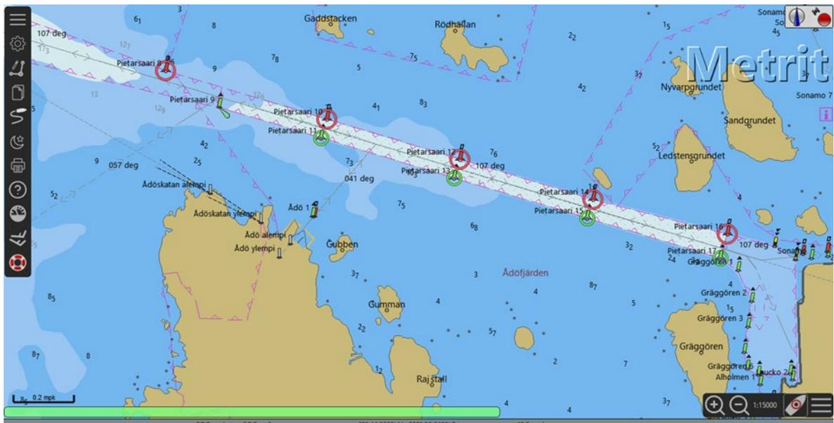
Fig.2. FI4EIJAJ cell on ECDIS before 30 March 2022 with 12,0 m Safety Depth setting.
