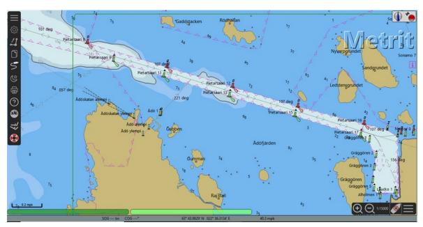
Fig. 3. FI4EIYAJ cell on ECDIS after 30 March 2022 with 12,0 m Safety Depth settings.
