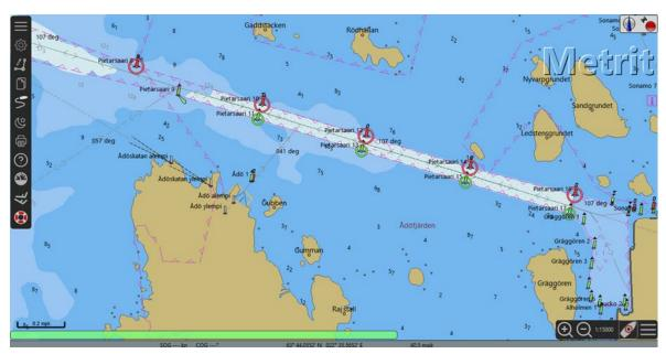
Fig.2. FI4EIYAJ cell on ECDIS before 30 March 2022 with 12,0 m Safety Depth setting.
