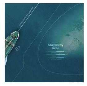
StayAway addresses the challenge of inadequate or outdated ENC data by providing digitized information on the precise location and extent of uncharted shallow obstructions.
