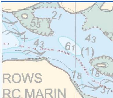
CSB filled in between systematic line spacing in a narrows giving a better limiting depth.
