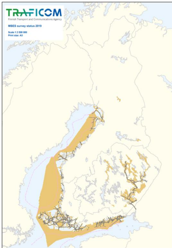
Fig. 2. Hydrographic re-survey coverage in 2019 surveyed according to IHO S-44 and FSIS-44 standards
