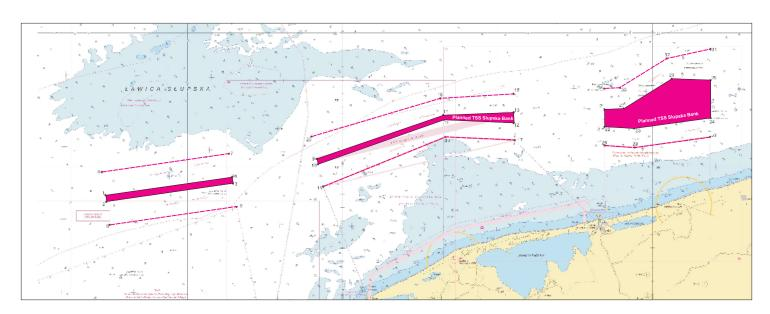
The existing eastern section of the *TSS "Slupska Bank"* is to be modified in such a way as to align its traffic lanes with the traffic lanes of the new section of the *TSS*.
