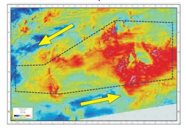
Having considered possible methods of reducing the risk of ship groundings in the area, the Polish Maritime Administration decided to establish a new section of the *TSS "Slupska Bank"* with two lanes designed to separate opposing traffic flows and to bypass the area of detected shallows where a traffic separation zone is to be established.
