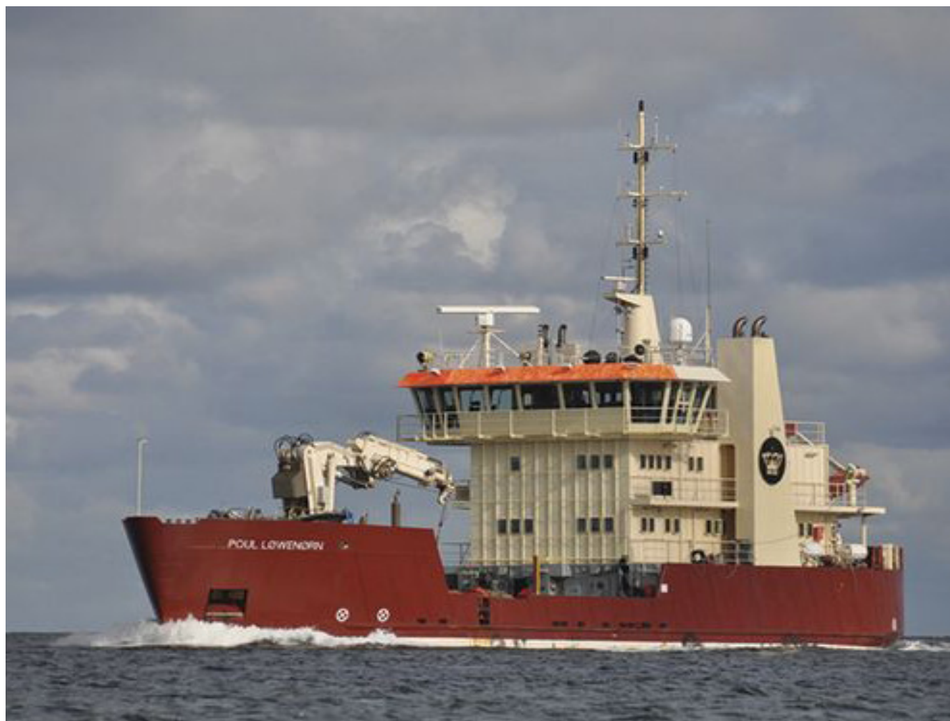
Figure 7: POUL LØWENØRN was fitted with two new cabins, a larger mess and was built 5 meters longer.
