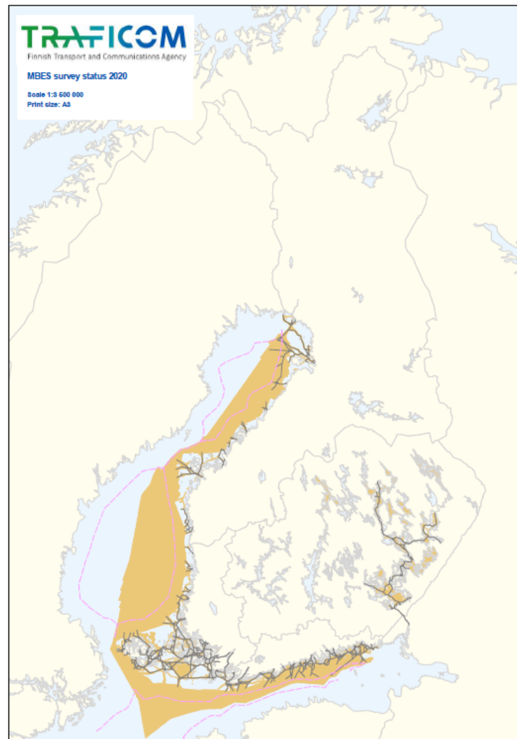
Fig.2. Hydrographic re-survey coverage in 2020 surveyed according to IHO S-44 and FSIS-44 standards.
