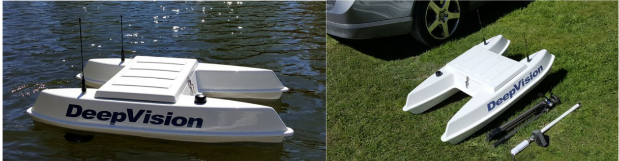
Figure 6 Surveying with ASV is tested with this system from Deep Vision. Pictures from Deep Vision.
