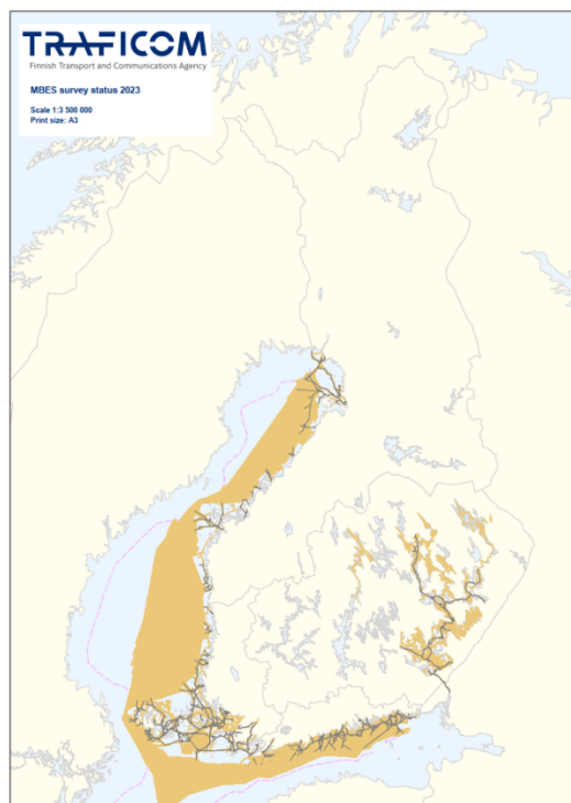
Fig.2. Hydrographic re-survey coverage at the end of 2023 surveyed according to IHO S-44 and FSIS-44 standards.
