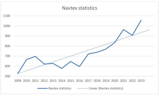
The statistics show an increasing number of warnings during 2023 reaching over 1000 for the first time. This is alarming when maintaining the 10-minute time-slots for the Navtex transmitters.
