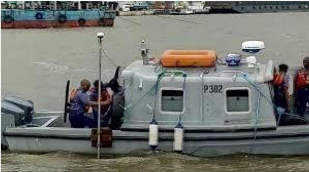
Figure 4. Specially modified EPENAL E-27 Survey Boat
