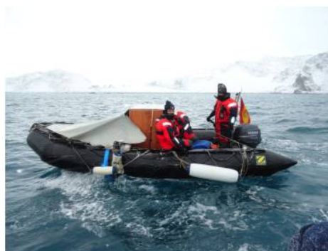
Figure 3. Very shallow water bathymetry system operated from a small rubber boat
