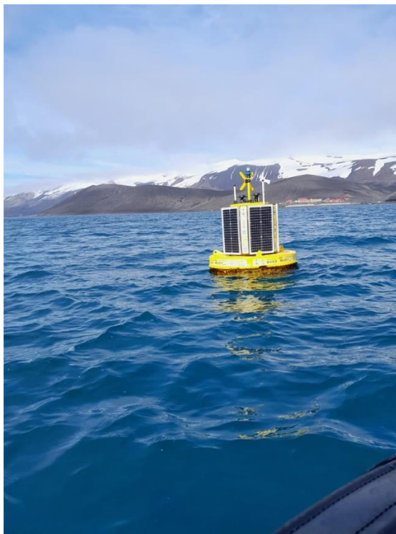
Figure 18. Bouy for measuring sea level in real time
