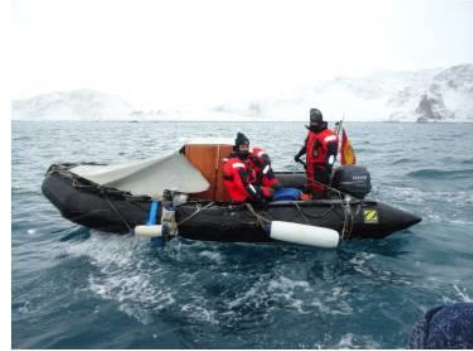
Figure 3. Very shallow water bathymetry system operated from a small rubber boat
