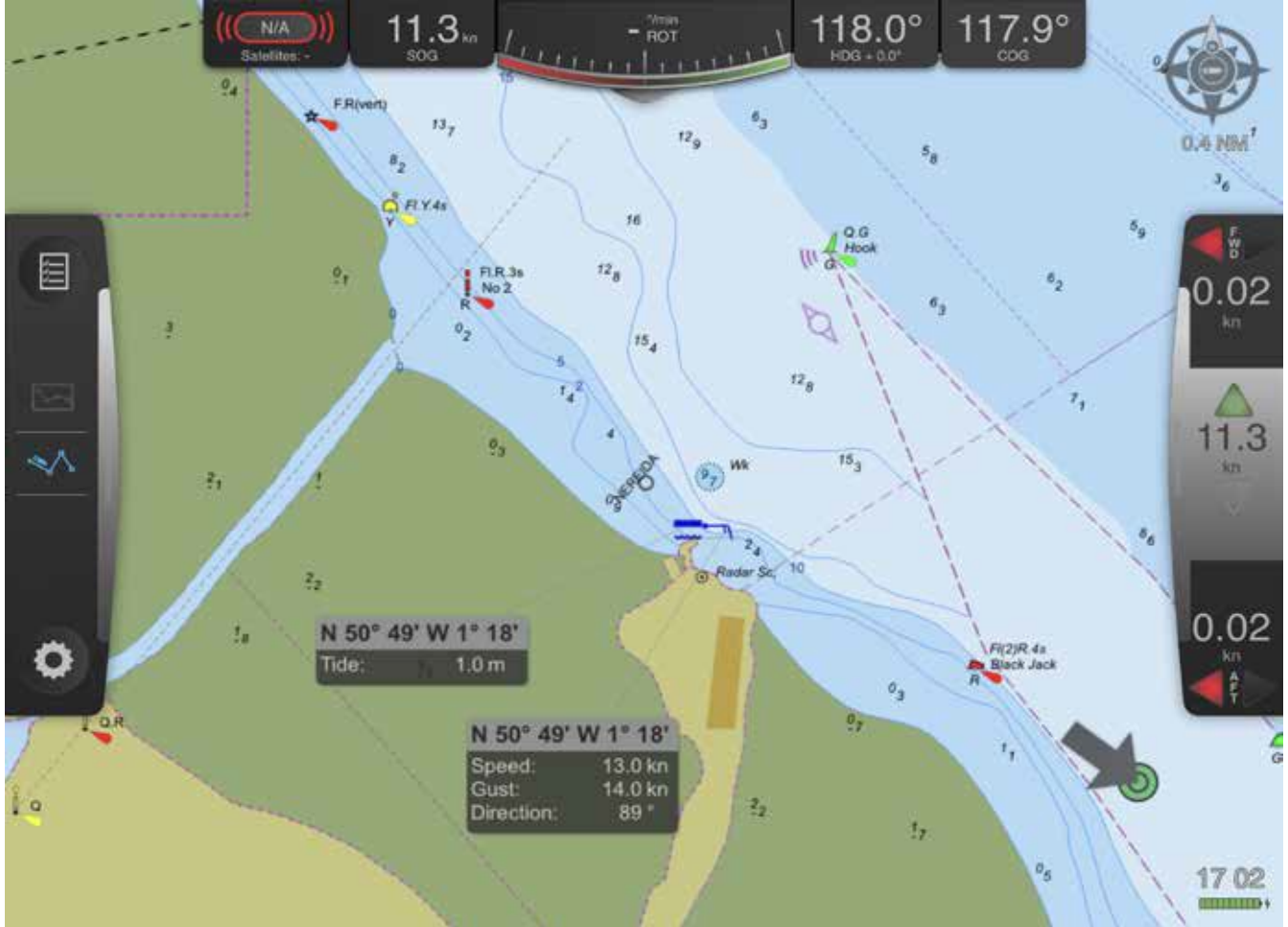
Screen shot example from a Trelleborg 'Safe Pilot' Portable Pilot Unit showing how maritime pilots use data including water depths, vessel tracks, weather and tide information.
