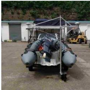
MBES Norbit iWBMSH integrated to Shom's deployable hydrographic system
