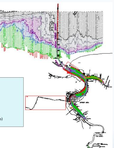
Channel depth 4.5 m (available since January 1<sup>st</sup> 2022) Average Springtide 2.8m Average Neap tide 2.15m Average Water depth Available at Springtide 7.3m Average Water depth Available at Neap tide 6.65m UCK ( not included , variable depending on ship) Channel depth 5.5 m (Start 15 okt. 2022) Average Springtide 2.8m Average Neap tide 2.15m Average depth Available at Springtide 8.3m Average depth Available at Neap tide 7.65m UCK ( not included , variable depending on ship)
