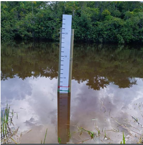
Figure 7: Local tide gauge with the flood mark (red line).
