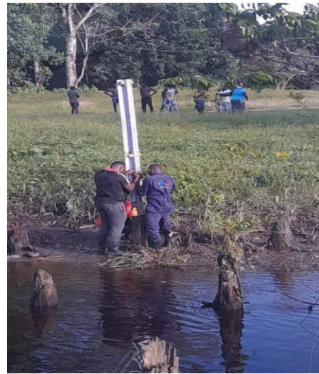
Figure 8: Set up of local tide gauge
