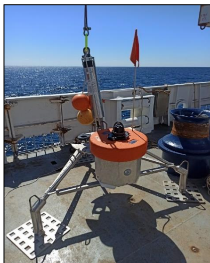
Fig. 6 – CATRINE frame mooring with its orange buoyancy above the canister
