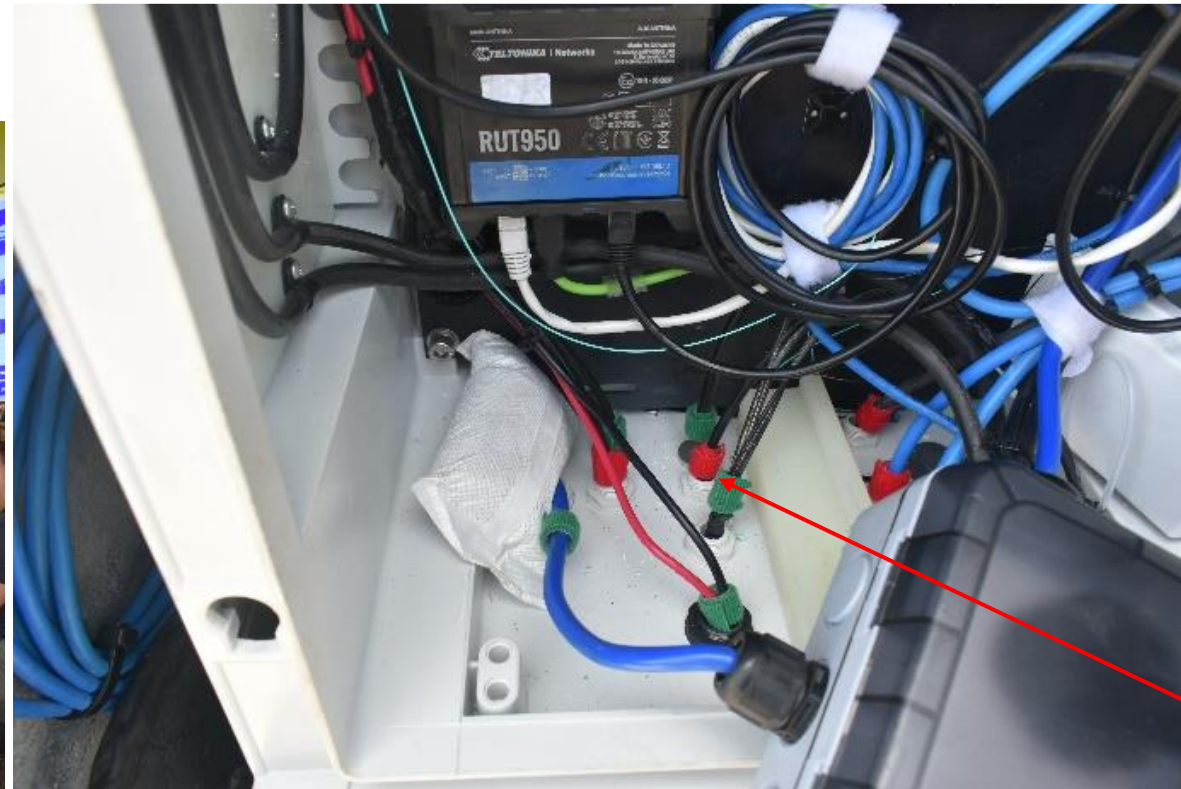
Cabling with red and green markings to assist with mast removal in the event of a storm
