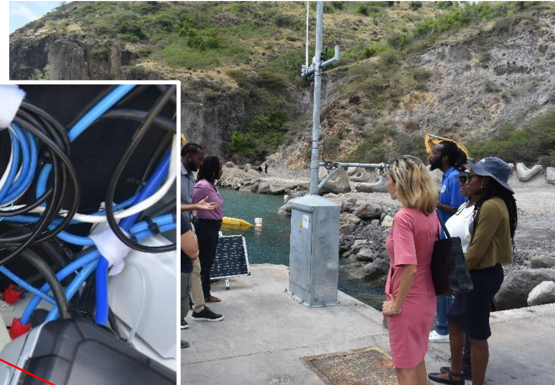
Cabling with red and green markings to assist with mast removal in the event of a storm
