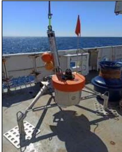
Fig. 1 – CATRINE frame mooring with its orange buoyancy above the canister
