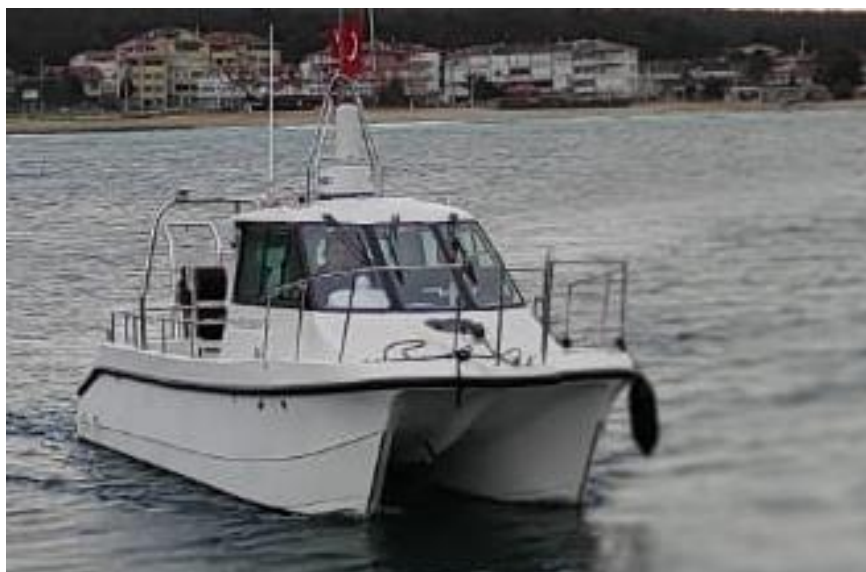
New catamaran type semi-autonomous survey boats
