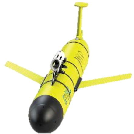
Figure 17. – UUV Slocum Glider G3
