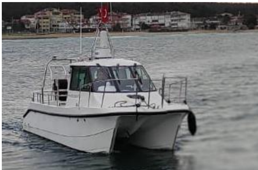
New catamaran type semi-autonomous survey boats
